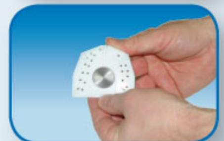
14. Fit the base plate with pins
