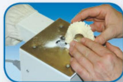
26. Saw the tooth crown with a diamond blade
