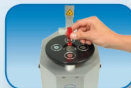
J. Carry out a test drilling and inspect the results after adjusting the settings
